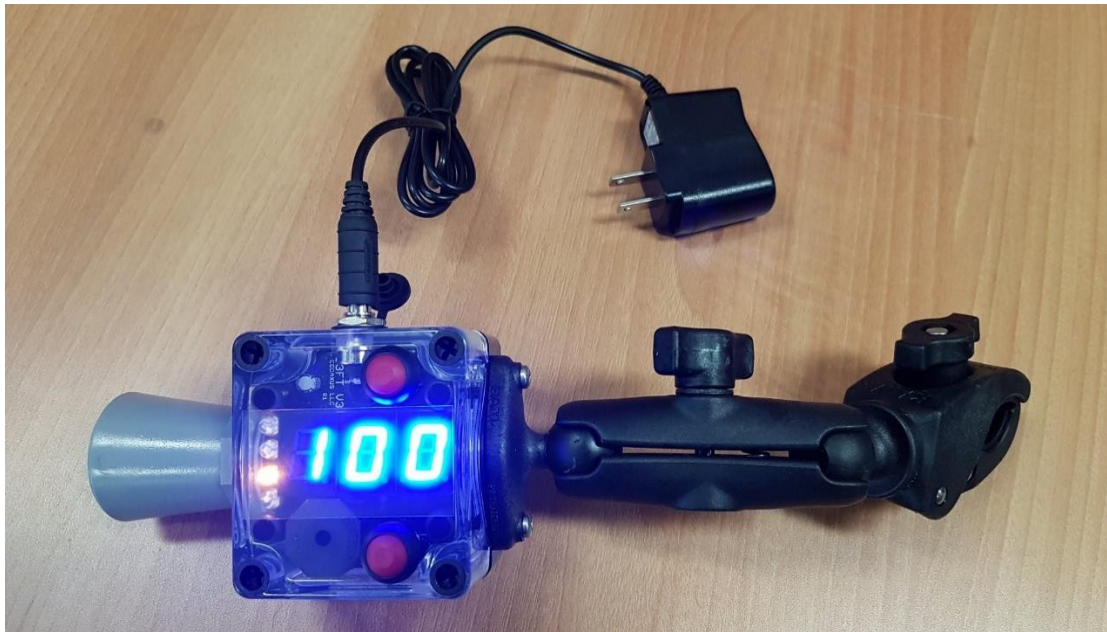
Figure 11 Guelph Police Service's one-meter measuring device.
